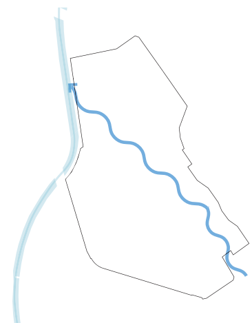
Figure 6: Open space should provide for an overland flow path and water sensitive urban design.
